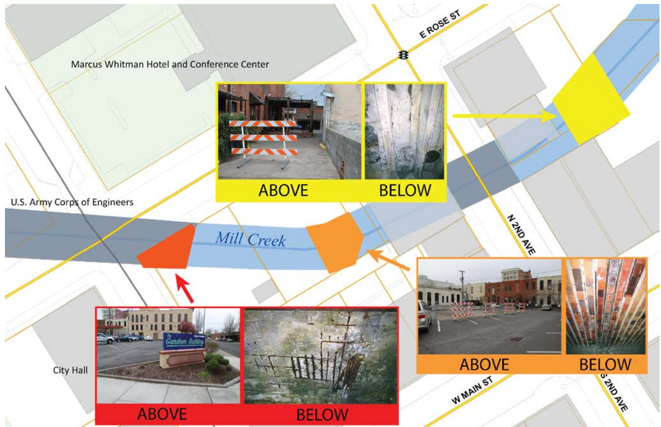
Figure 2.4-16. Downtown Walla Walla Non-Bridge Structures Rated in Poor Condition (Olson 2016)
