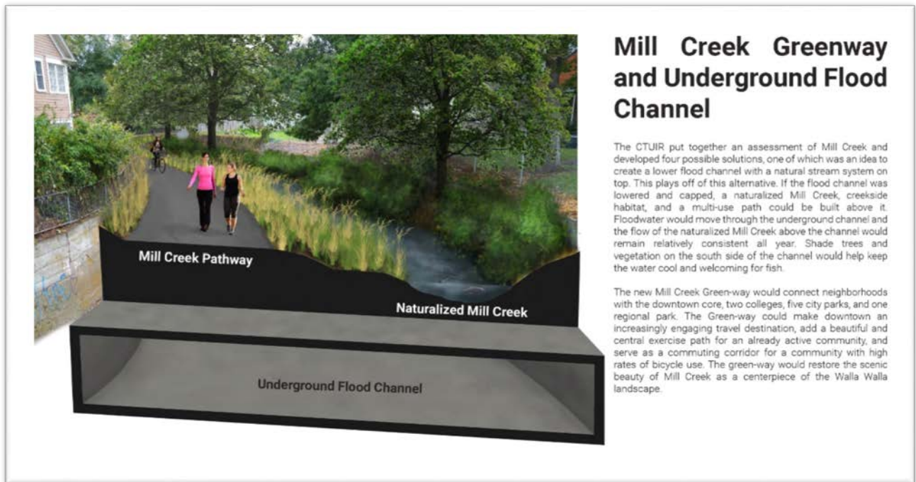
Figure 5.3-6. Visualization of Underground Flood Conveyance Conduit (WSU 2016b)
