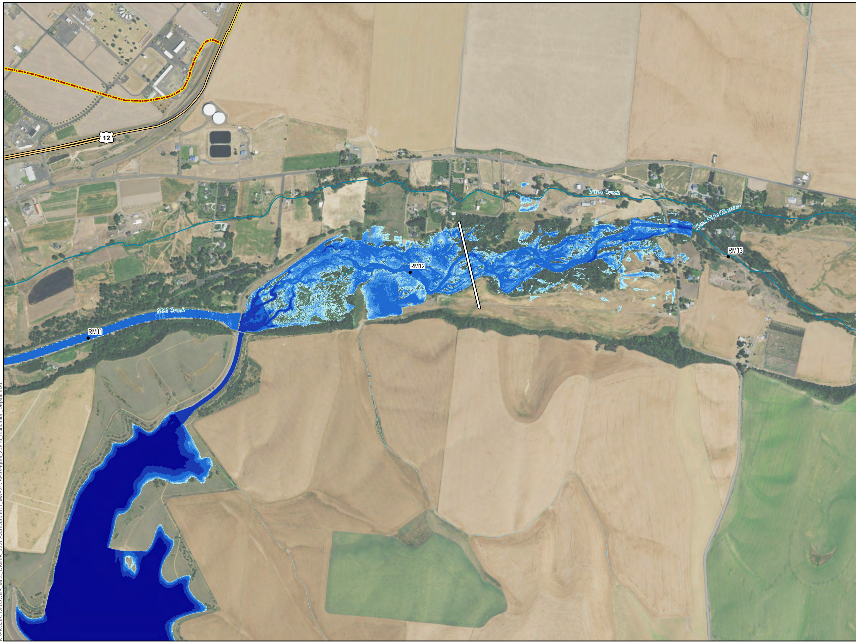
FIGURE 2.5-21 INUNDATION MAP OF 1996 MILL CREEK FLOOD 3,500 cfs Bennington Diversion Dam
